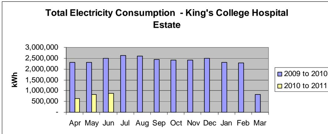
Imported electricity consumption reduced considerably on the main hospital site from March 2009. This was the result of the start of the operation of the combined heat and power plant (CHP) on 3<sup>rd</sup> March 2009.
